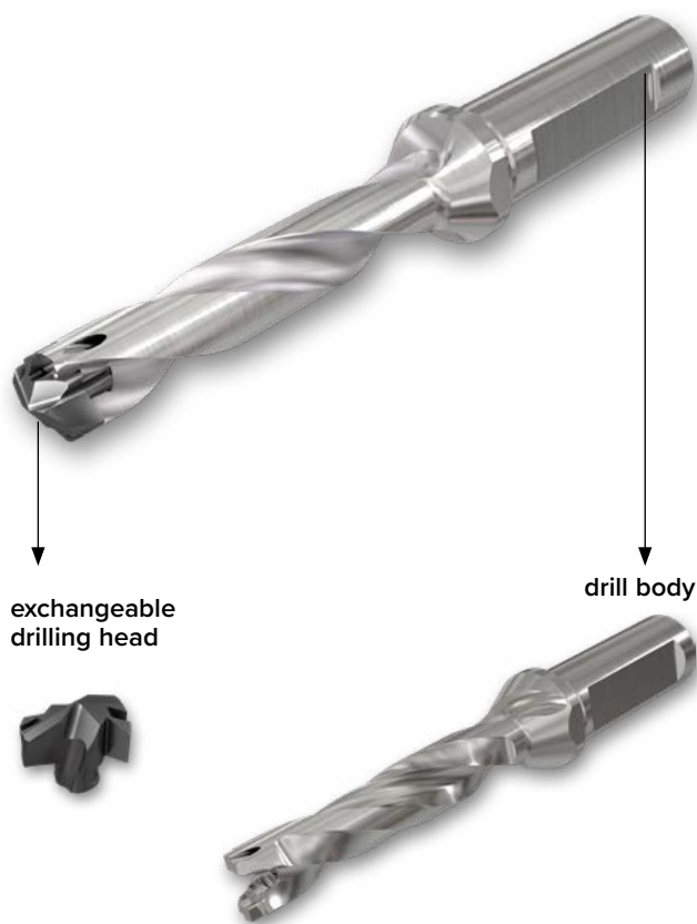
exchangeable head drill
